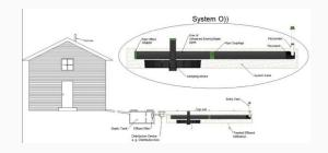
System O)) is a treatment system. As per the Ontario Building Code Section 8.9.2.4., all treatment systems require annual sampling. System O)) is equipped with a sample device and port that make it very easy to acquire a sample. Remember-the sample device must be installed at the front of the system, on the header side.
