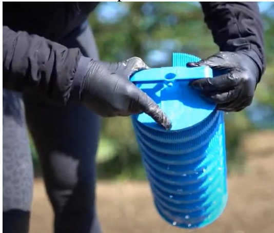
Figure 6. Arrow on the effluent filter
