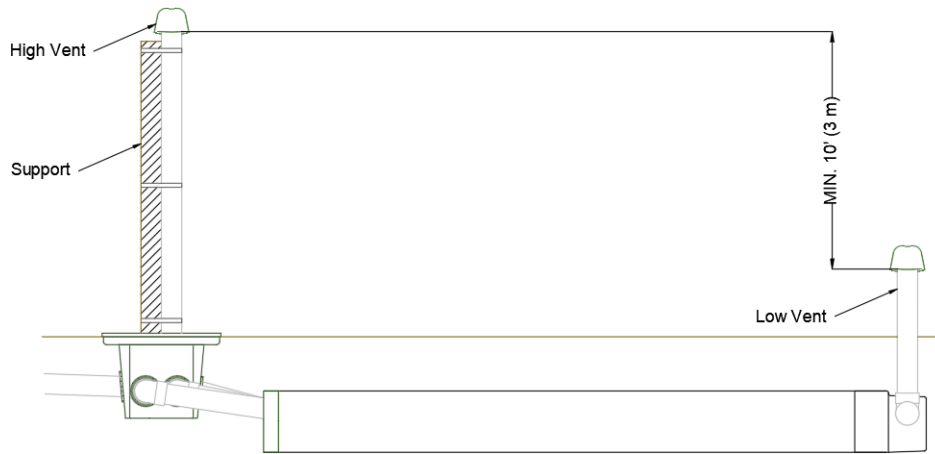
Figure 46. Differential venting – Standard configuration
