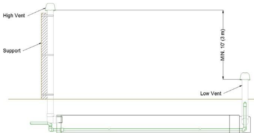
Figure 47. Differential venting – Low-pressure Distribution for Standard Configuration
