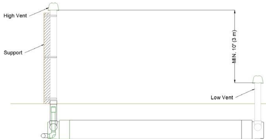
Figure 47. Differential venting – Low-pressure Distribution for Standard Configuration
