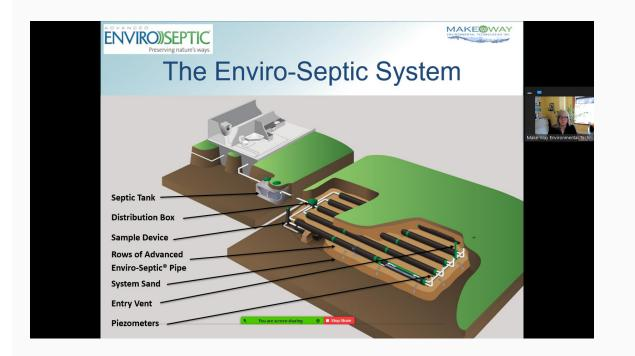
The Enviro-Septic System is a simple and easy septic system, producing Level IV Quality Effluent.
